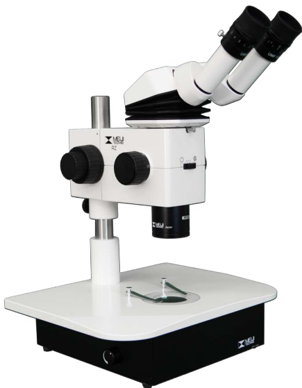
MA749: Ergonomic viewing head MA730: UWF 10X eyepieces (2) RZ-B: 10:1 Zoom body with built-in dual iris diaphragm and click stops MA742: 1.0X Plan Achromat objective RZBD/LED: Brightfield/Darkfield LED transmitted light stand
